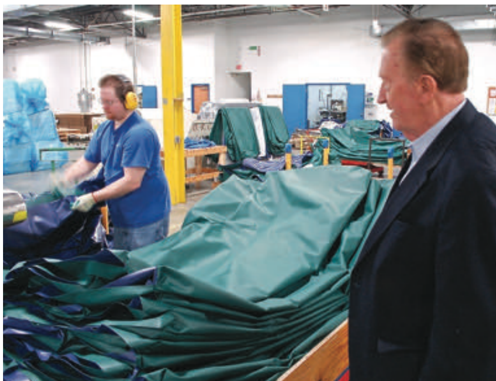
In the manufacturing plant, Bob Barker watches an employee assemble mattresses with welded seams for sanitation and safety purposes in prisons. A vacuum Bob helped develop reverses the covers at this stage.
