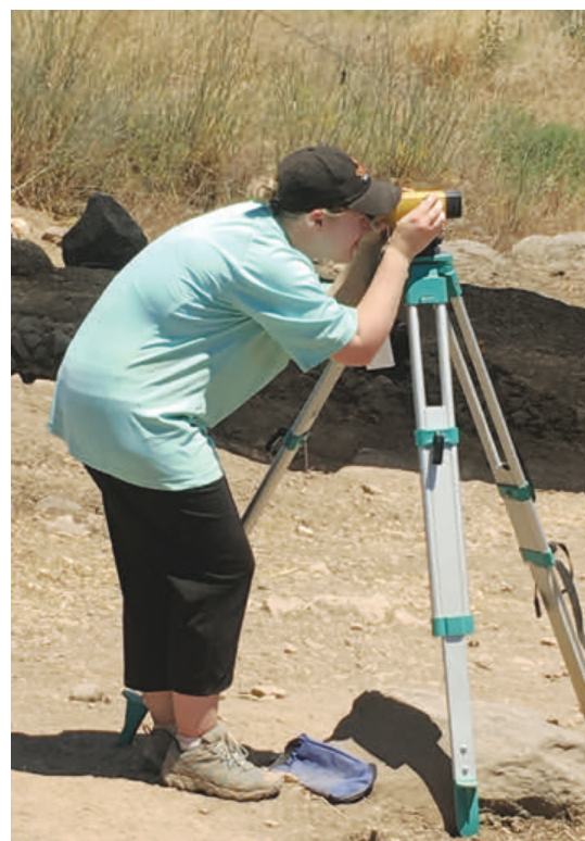
CHECKING — Muriel Lasater, both student and Assistant for Financial Aid at CUDS, using a “Dumpy” to measure the level of a find inside the square.
