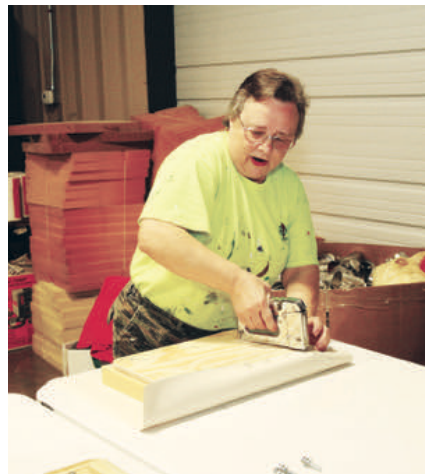
PRODUCTION CYCLE — Volunteer Susan Keene staples upholstery to the seat bottoms and backs of the mobility carts manufactured by the Huntsville, Ala., nonprofit. The carts, produced in a new, state-of-the-art facility, are built to withstand extensive use in remote parts of the world.
